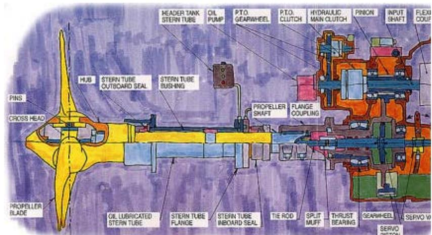
Actuation of the pitch is done through a mechanical connection from the blades to a hydraulic actuation system inside the gearbox (push-pull rod through the propeller shaft).
