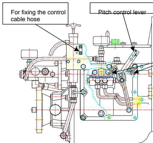
Adjust the cable so that the pitch control lever o gearbox are on top whe the pitch control lever o bridge are in the same position.
