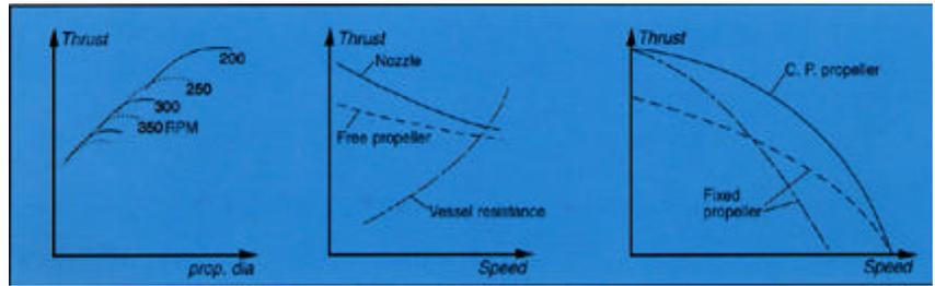
A fixed propeller designed for maximum speed can not give power at low speed. Conversely, a fixed propeller designed for power can not give maximum speed. A controllable pitch propeller, however, gives both maximum speed and maximum power.
